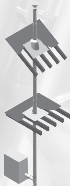
Secure Seal Double Wall (SSD) Vertical Through-the-Roof Installation
