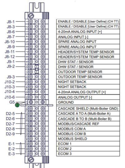
**Enable/Disable**  $-\underline{TB1-1}$  and  $\underline{TB1-2}$  can be used to remotely enable or disable the boiler. The functionality of these terminals is user-configurable through the NURO<sup>®</sup> controls, but generally closure of the Enable/Disable circuit provides a call for heat to the boiler. Opening this circuit prevents the boiler from running.
