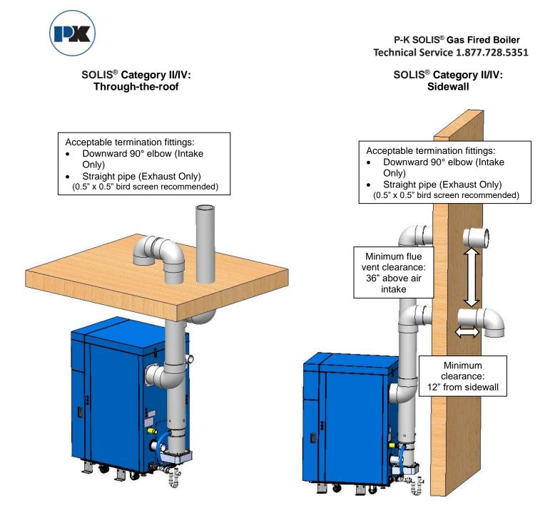
**NOTE:** For **Category II** installations, ensure the flue venting system is designed to maintain a slightly negative exhaust pressure **between -0.01**" **W.C. and -0.05**" **W.C.**
