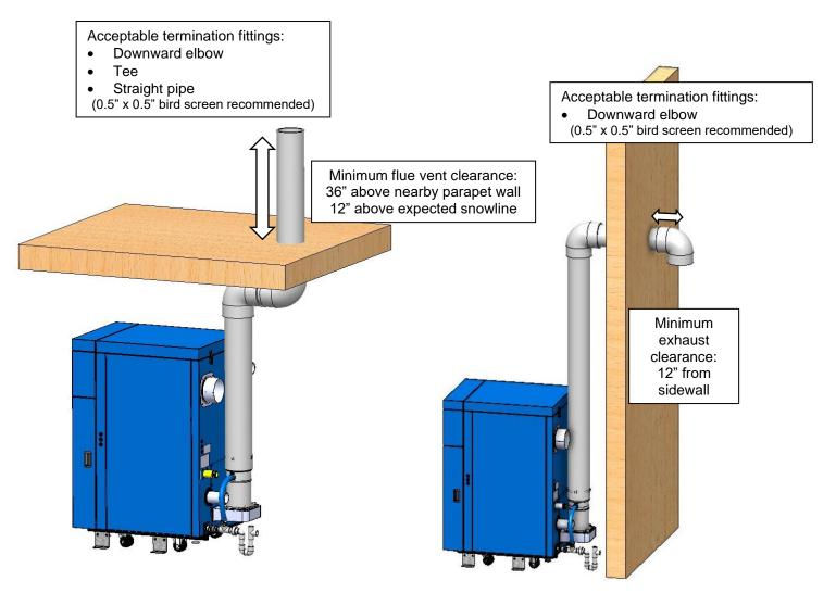
**NOTE:** For **Category II** installations, ensure the flue venting system is designed to maintain a slightly negative exhaust pressure **between -0.01**" **W.C. and -0.05**" **W.C.**
