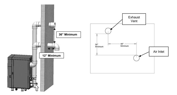
The combined pressure drop of the air supply duct and exhaust vent must not exceed 0.7" W.C. This pressure drop includes both the inlet and exhaust duct friction loss. If the air inlet and the exhaust vent terminate on the same wall of the building, they must utilize the same type of termination fitting. Allowable termination fittings are either 90° elbows or tees. This boiler may be installed with sidewall vent using room air, see 3.4.1.
