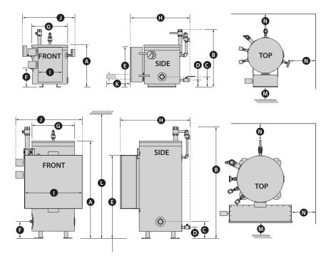
FIGURE 1 - BOILER DIMENSIONS
