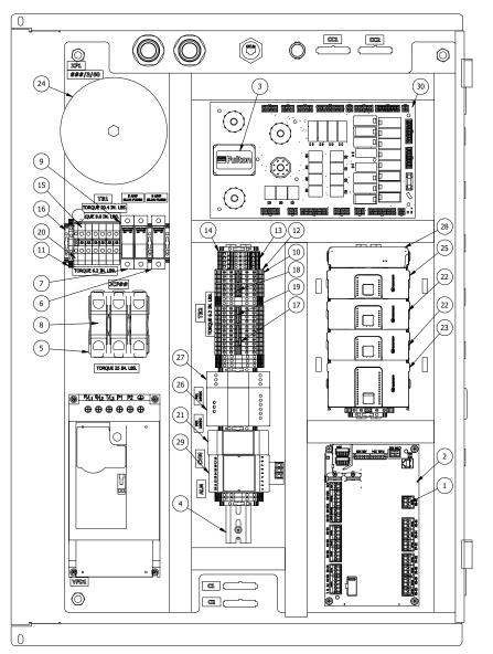
FIGURE 33 - ELECTRICAL CONTROLS EDR+ 2500 - 3000
