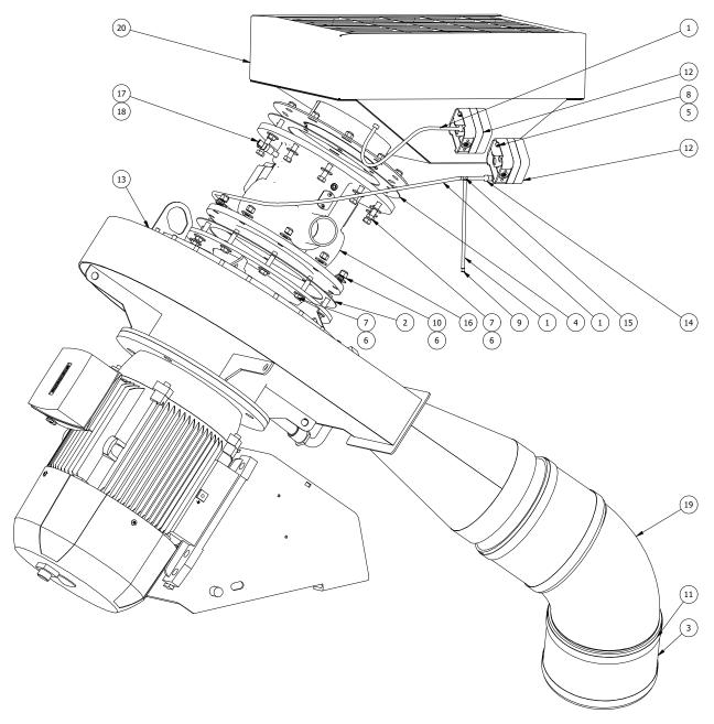
FIGURE 37 - PRE-MIX ASSEMBLY EDR+ 6000
