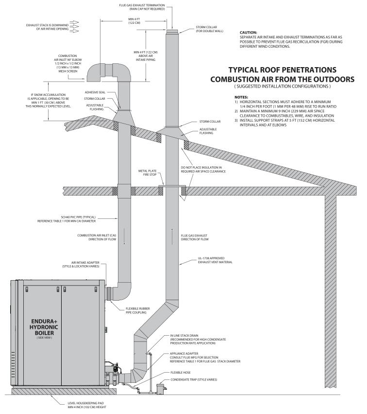
FIGURE 19 - ROOF PENETRATION DETAILS
