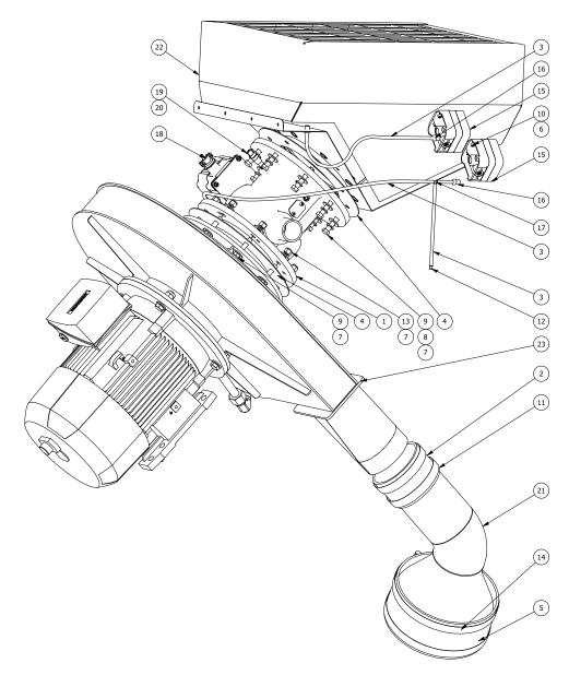
FIGURE 36 - PRE-MIX ASSEMBLY EDR+ 4000 - 5000
