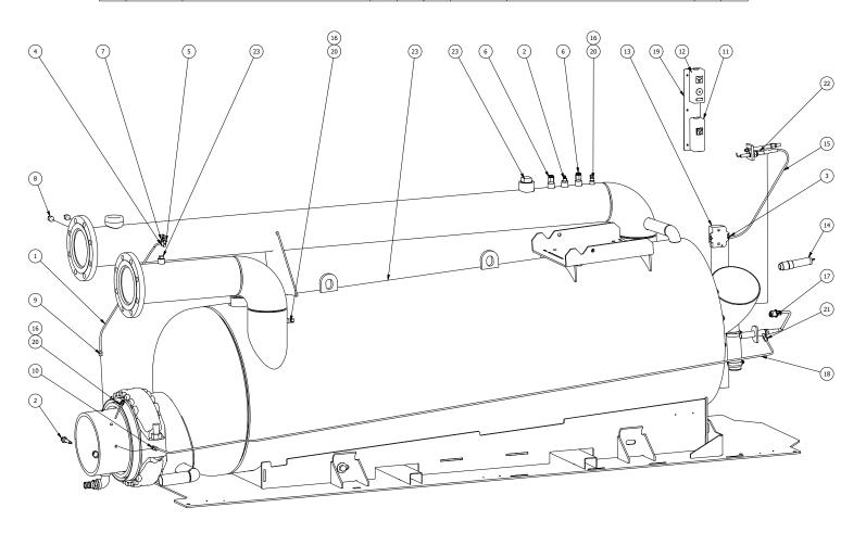
FIGURE 29 - INSTRUMENTATION AND DEVICES EDR+4000-6000
