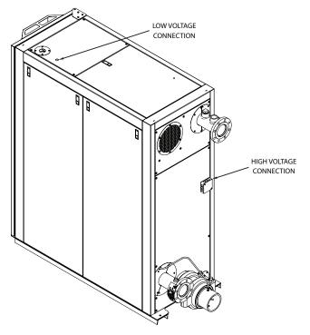
FIGURE 25 – HIGH VOLTAGE AND LOW VOLTAGE CONNECTION LOCATIONS (TYPICAL)
