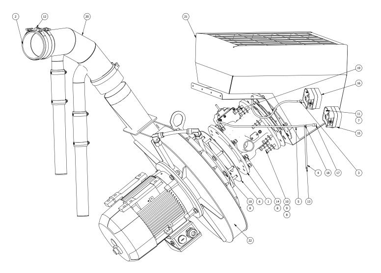
FIGURE 35 - PRE-MIX ASSEMBLY EDR+ 2500 - 3000
