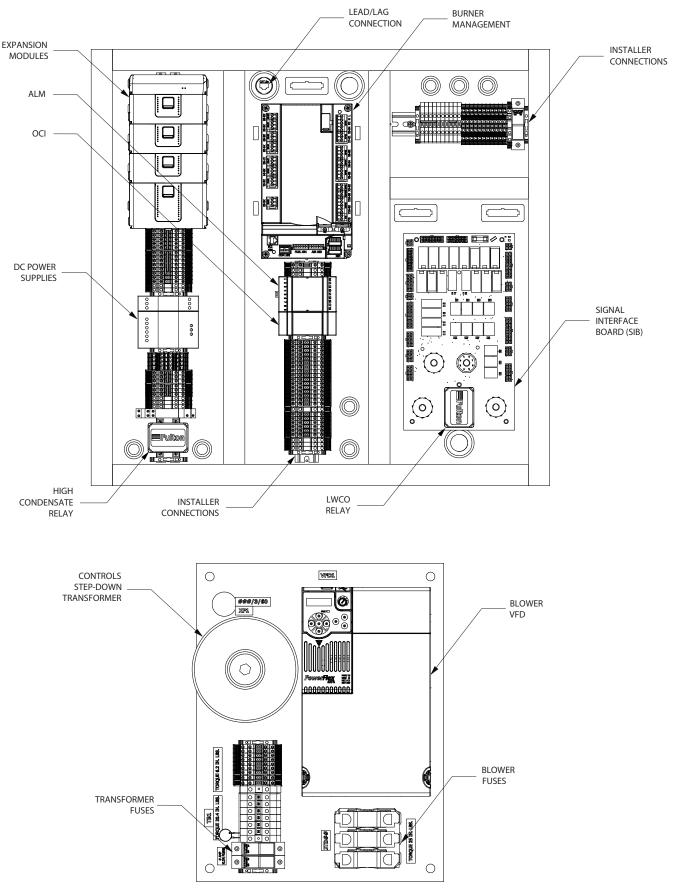
FIGURE 24 - EDR+4000-6000 ELECTRICAL CONTROLS LAYOUT
