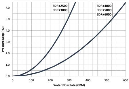
FIGURE 3 - TYPICAL WATER SIDE PRESSURE DROP
