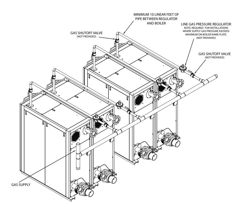
FIGURE 10 - ENDURA+ MULTIPLE BOILER GAS SUPPLY PIPING
