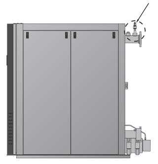
FIGURE 2 - SAFETY VALVE INSTALLATION LOCATION
