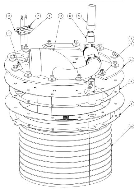
FIGURE 38 - BURNER EDR+ 2500 - 3000
