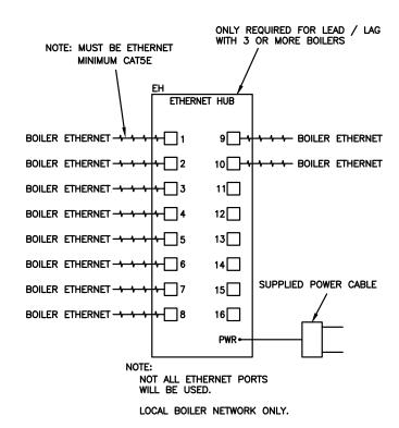
FIGURE 26 - ETHERNET-IP FIELD WIRING
