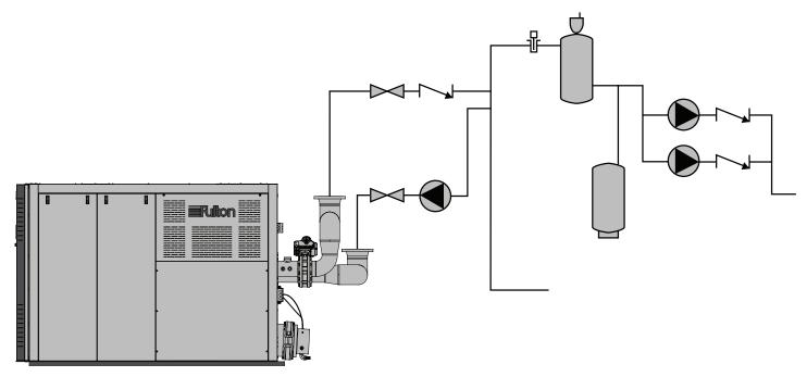
FIGURE 6 - SAMPLE PIPING LAYOUT, PRIMARY - SECONDARY PIPING; SINGLE BOILER
