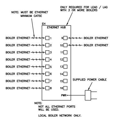
FIGURE 22 - ETHERNET-IP FIELD WIRING
