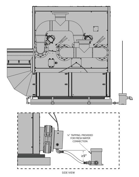
FIGURE 10 - CONDENSATE DRAIN PIPING
