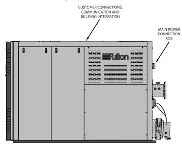
FIGURE 21 - ELECTRICAL CONNECTION LOCATIONS (TYPICAL)
