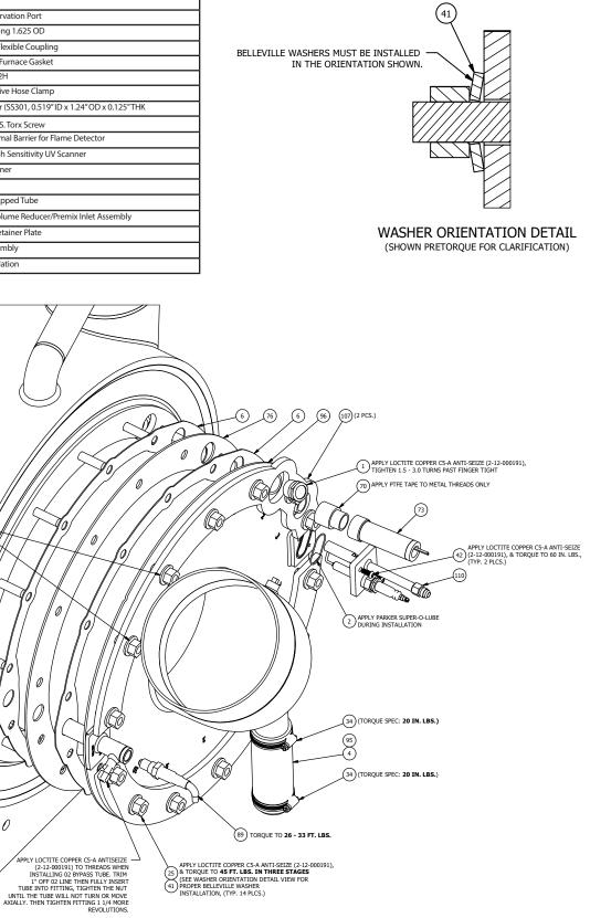
APPLY LOCTITE COPPER C5-A ANTI-SEIZE (2-12-000191), (25) & TORQUE TO **45 FT. LBS. IN THREE STAGES** (4) GEE WASHER ORIENTATION DETAIL VIEW FOR 1) PROPER BELEVILLE WASHER INSTALLATION, (TYP. 14 PLCS.)
