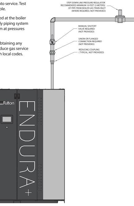
FIGURE 9 - FIELD GAS SUPPLY PIPING
