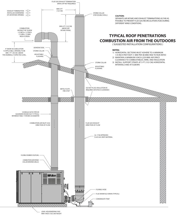
FIGURE 15- ROOF PENETRATION DETAILS
