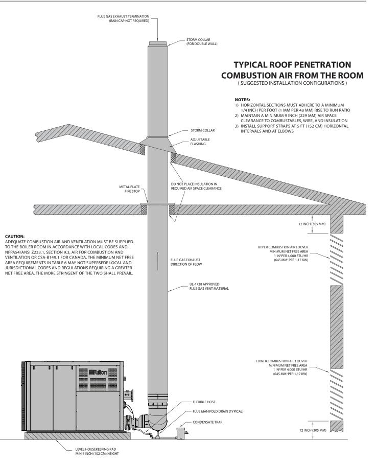
FIGURE 16 - ROOF PENETRATION WITH COMBUSTION AIR LOUVERS DETAIL
