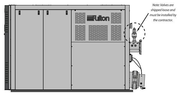
FIGURE 2 - SAFETY VALVE INSTALLATION LOCATION
