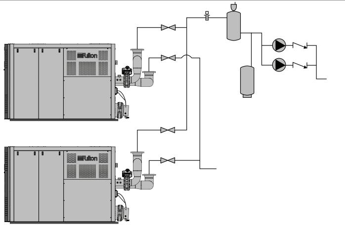
FIGURE 5 - SAMPLE PIPING LAYOUT, PRIMARY ONLY VARIABLE FLOW PIPING; MULTIPLE BOILERS
