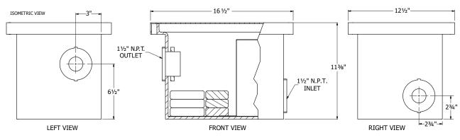
FIGURE 12 - FULTON PH NEUTRALIZING KIT
