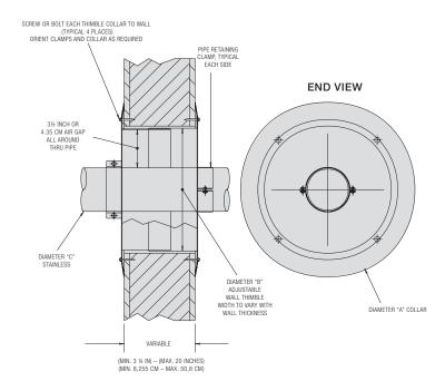
FIGURE 18- WALL THIMBLE INSTALLATION
