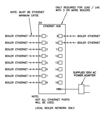
FIGURE 27 - ETHERNET-IP FIELD WIRING FOR 2-45-315010
