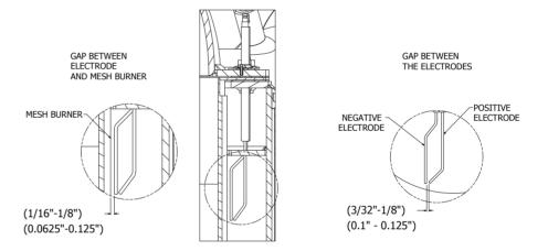
FIGURE 28 - IGNITOR GAP TOLERANCES
