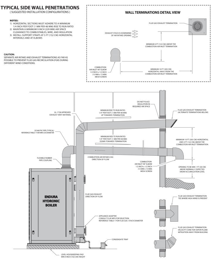
FIGURE 24 - SIDEWALL PENETRATIONS DETAIL
