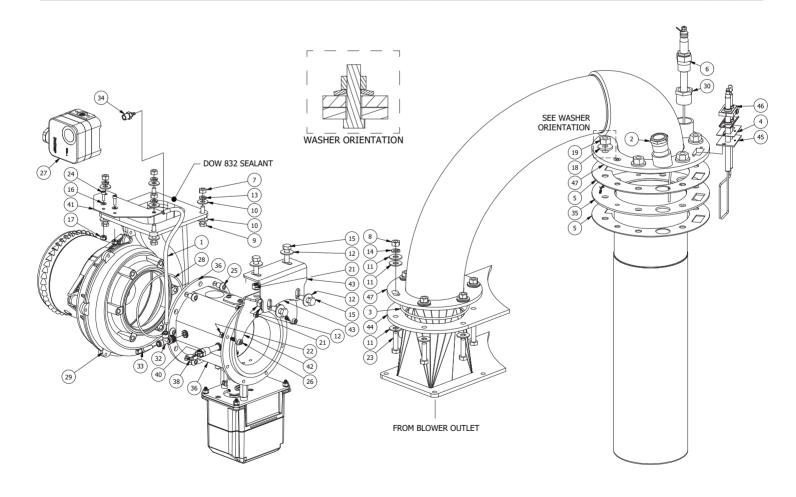
FIGURE 34 - BURNER AND PRE-MIX ASSEMBLY (EDR-750/1000)
