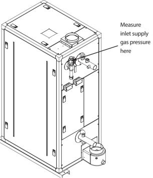
FIGURE 9 - MEASURING INLET GAS PRESSURE
