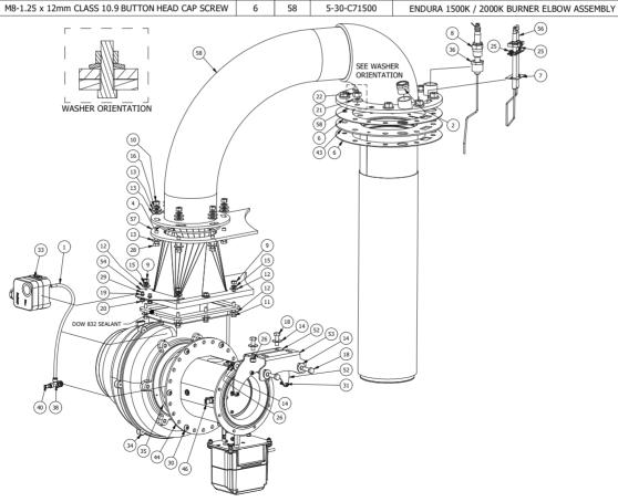
FIGURE 35 - BURNER AND PRE-MIX ASSEMBLY (EDR-1500/2000)
