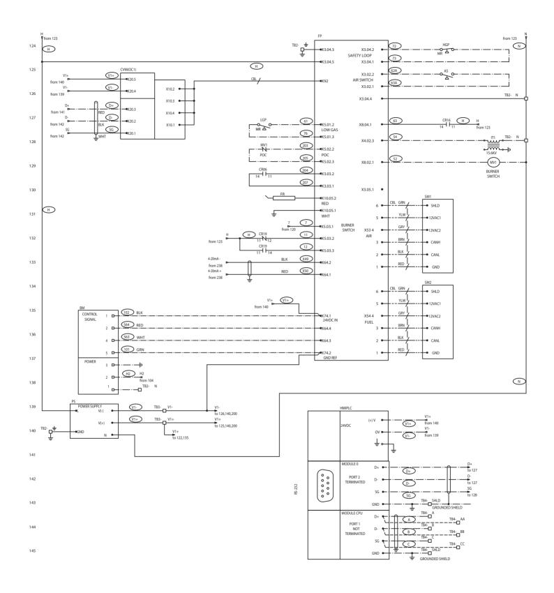
EDR 750 - 2000 PURE CONTROL REFERENCE ONLY ELECTRICAL SCHEMATIC DIAGRAM (CONTINUED)
