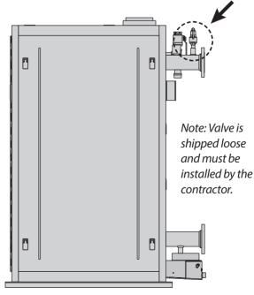
FIGURE 2 - SAFETY VALVE LOCATION
