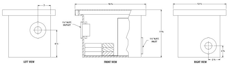
FIGURE 17 - FULTON PH NEUTRALIZING KIT
