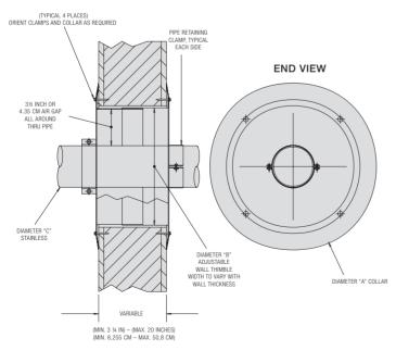
FIGURE 21- WALL THIMBLE INSTALLATION
