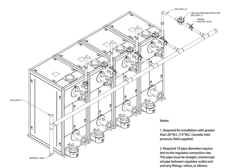
3. The line regulator should be installed with a minimum of 10 linear feet of pipe between the regulator outlet and boiler fuel train inlet.
