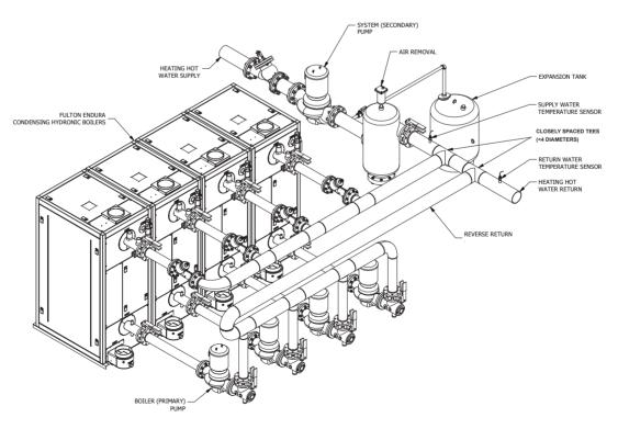
FIGURE 7 - SAMPLE PIPING LAYOUT, PRIMARY - SECONDARY PIPING; MULTIPLE BOILERS
