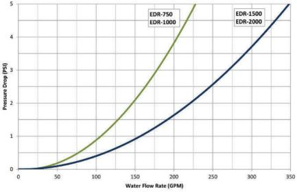
FIGURE 3 - TYPICAL WATER SIDE PRESSURE DROP
