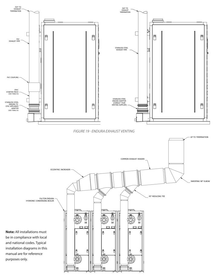
FIGURE 20 - ENDURA COMMON EXHAUST VENTING; TYPICAL INSTALLATION GUIDELINES
