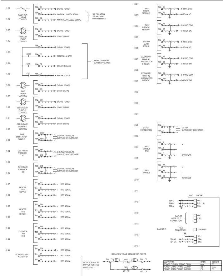
EDR 750-2000 PURE CONTROL REFERENCE ONLY FIELD CONNECTIONS
